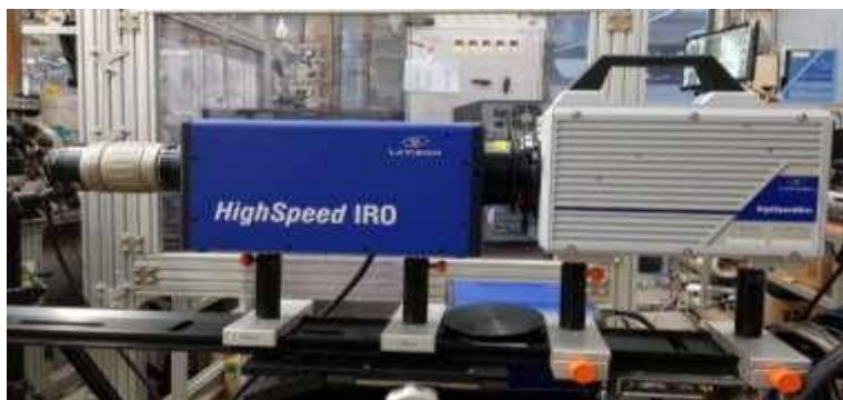
Figure 2. OH* Chemiluminescence experiment setup
